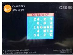
6. Stop charging, the battery voltage will goes down because of self-discharge, if need maintain battery voltage, please setup the **Restart Charge** YES (only for
